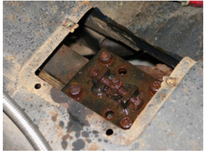
Detail of the device used to centre the rear transverse leaf spring.
