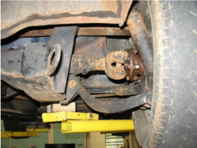
A detail of the rear suspension. Note the purposely bent lower a-arm and the non-rotoreflex u-joint configuration.
